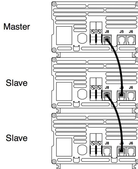
*Master–slave connections. The first unit must be
