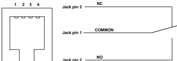
Common is connected to NC when the power is switched off.
