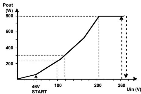
Output power / input voltage de-rating characteristic
