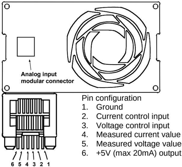
*Pin configuration of the modular connector J1
