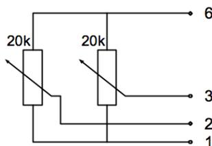
*Connecting example using the internal +5Vdc supply and external potentiometers.*
